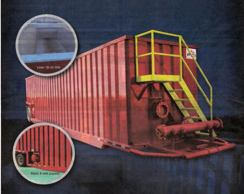
At **PCI Manufacturing**, quality paints and coatings ensure maximum performance from our tanks. That's why we cover the outside with high-solids Strathmore paint and the inside with a Carboline epoxy coating, while the undercarriage is
